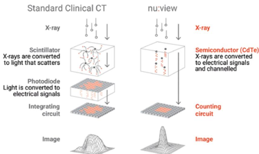
Comparison of the principle of standard clinical CT with that of single photon-counting detection. The single photon-counting detector provides excellent image quality at low dose
